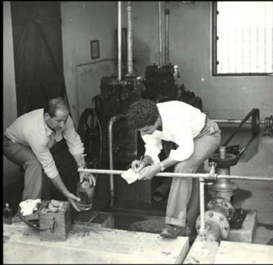
This is the bacteria test. We had ice inside the sterilized bottle and we burnt the tap to get rid of the bacteria
